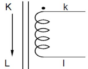
Figure 2. Schematic of the Current Transformer
