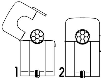
**⚠ Important:** Secondary side cables must be connected to KES Plus (keeping polarity) before closing the clamp to the primary side cable.
