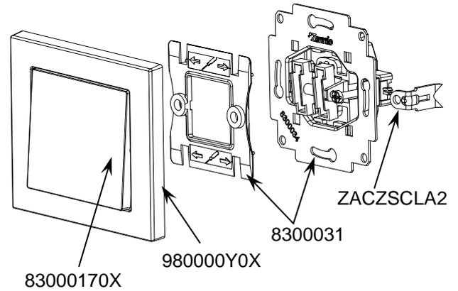
Figure 1. Single two-way rocker switch
