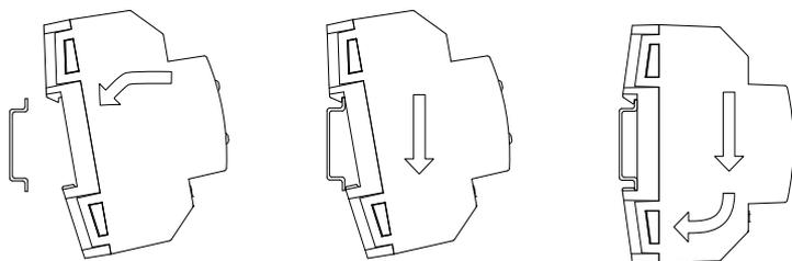
Removing DIMinBOX DX1 from DIN rail:
