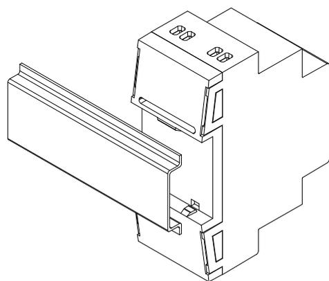
Figure 3: Mounting DIMinBOX DX1 on DIN rail
