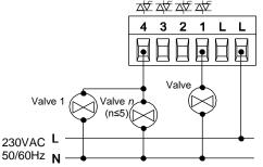
• NOTE: Simultaneous connection of one valve to several outputs is not allowed.
