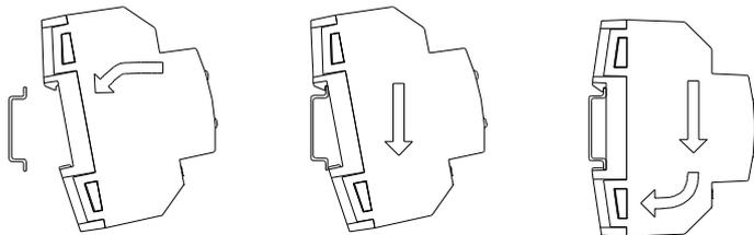
Removing HeatingBOX 24V 4X from DIN rail:
