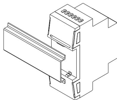
Figure 3: Mounting HeatingBOX 24V 4X on DIN rail
