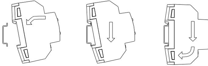
Removing KIPI from DIN rail:
