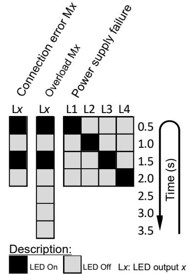
Figure 2: Error notification through grille status LED
