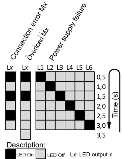
Figure 2: Error notification through grille status LED
